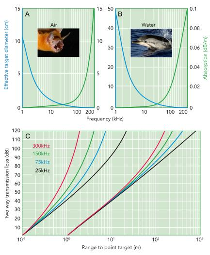
FIGURE 2. Target size that generates geometric backscatter and absorption
